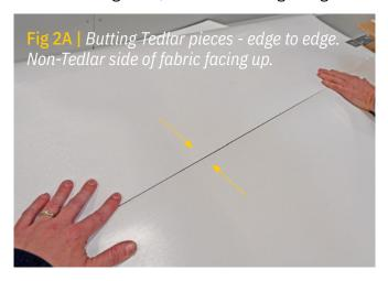
Then take a third piece of *NON*-Tedlar fabric, cut into a 2" to 6" strip, centered over the joint of the first two pieces, and weld with a wide bar.
