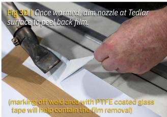
The melting will happen quickly and the Tedlar film will roll back on the surface of the PVC coating. You can work along the area that need to be welded, removing the Tedlar film.
