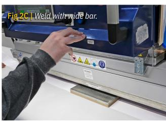
Care should be taken to keep the bottom two pieces from coming apart in the welding process. This method of welding is very useful when splicing the end of one roll of material to the beginning of a second roll of material.
